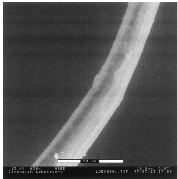
Figure 2 Elementary flax fibre which has just developed a kink band.
